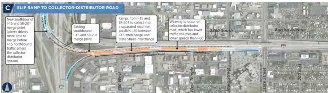
Figure 8 Alternative C: Slip Ramp to CD Road
