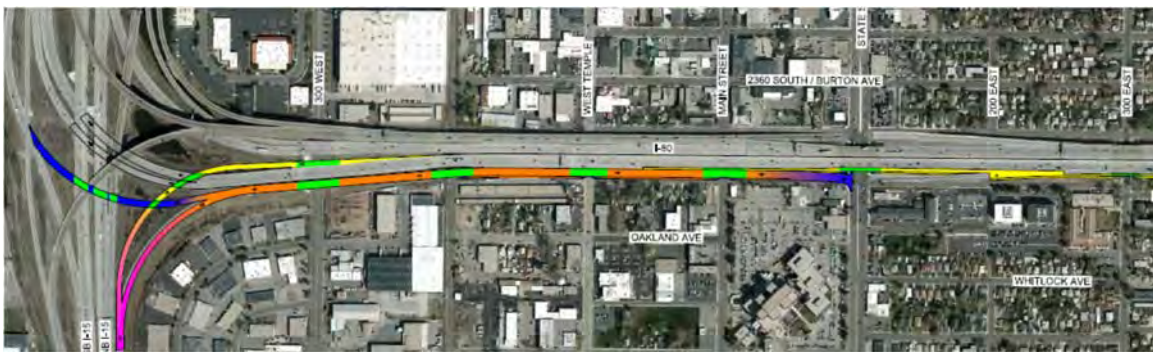
Figure 14 Alternative H: CD System to State Street, I-15 NB Flyover, Additional EB Lane
