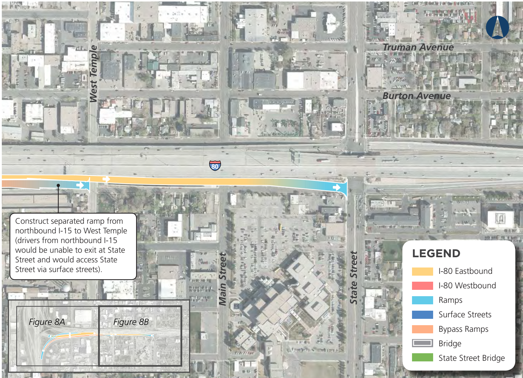
Figure 8B Eastbound Weave Alternative F – I-15 NB to West Temple with Flyover
