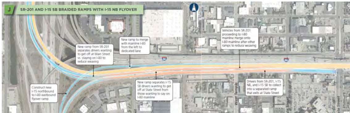
Figure 16 Alternative J: SR-201 and I-15 SB Braided Ramps with I-15 NB Flyover
