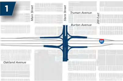
SINGLE POINT URBAN INTERCHANGE (SPUI)
