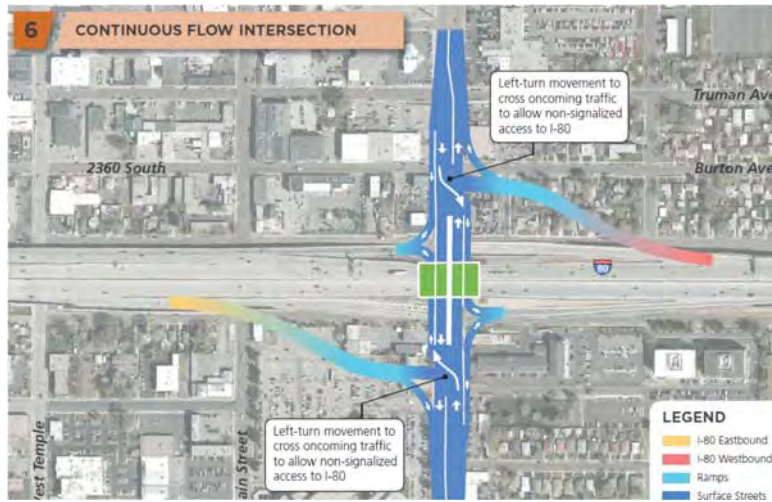
Figure 29 Alternative 6: Continuous Flow Intersection
