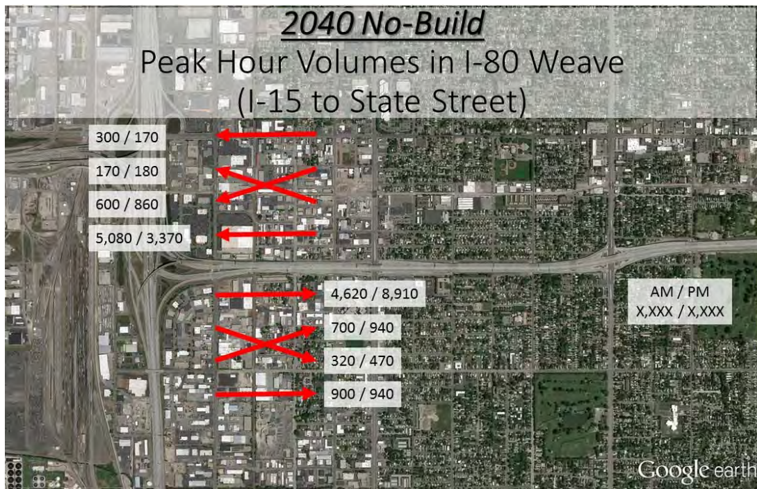
Figure 3 I-80 Weave Sections East- and Westbound
