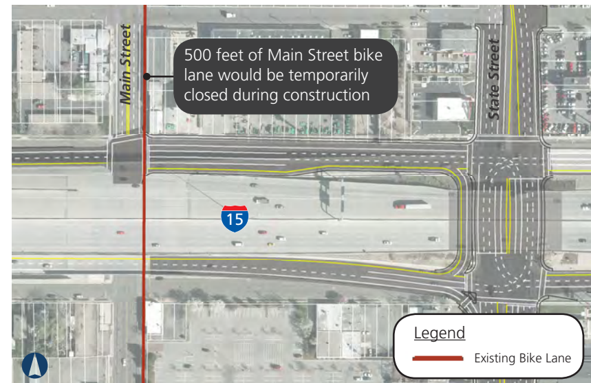
Figure 3-21 Interchange Alternative 3N Bike Lane Impacts
